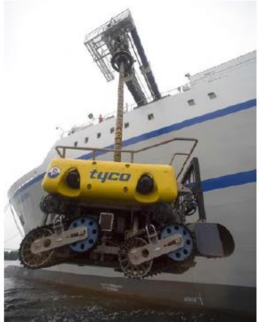
ROV used for cable inspection, recovery and burial
